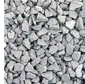
Recycled concrete aggregate Floor slabs
